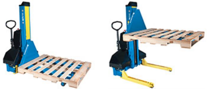
The UniLift's power is provided by an efficient 24 VDC battery system and on-board, automatic battery charger. It also features electro-mechanical outrigger actuation with position sensors. This leads to a lower energy usage, which in turns saves your company the cost of a high electric bill.
