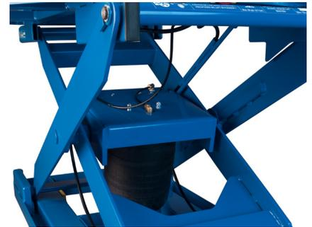
The EZ Loader's self-contained pneumatic system eliminates the need for a constant air connection, thereby eliminating the need for mechanical springs.
